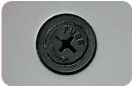
The fuse holder is located on the bottom of the device.
